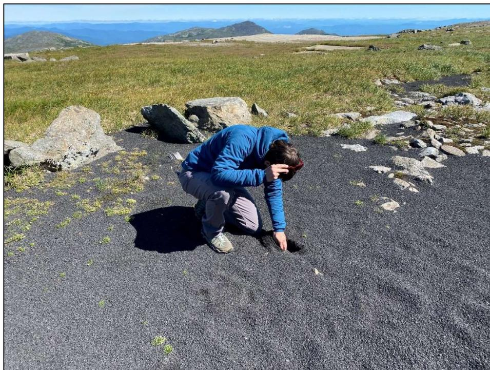
**Photo 4.** Hand excavating to determine depth of coal sediment deposit.
