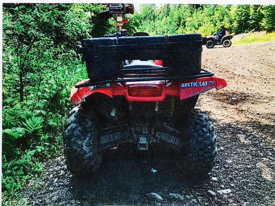
8. View from rear of ATV; visible damage to plastic, rack, and storage box.
