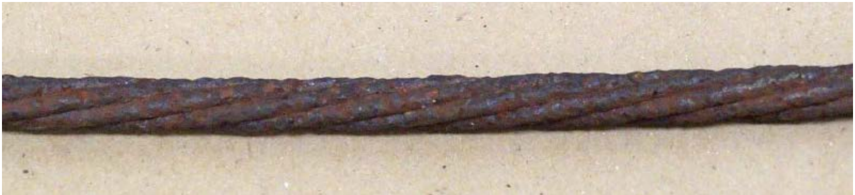
Severe Corrosion of 3/8 Shield Wire Sample
