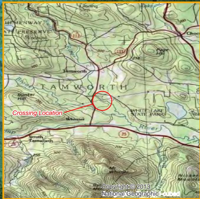
Public Water as shown below in Map identified in the application and engineering drawings as State of New Hampshire and located in Tamworth. The project will require the Department to grant a license for the 115 kV transmission line from Structure 237 east to Structure 238. This crossing spans 739.2 feet with 61.3 feet crossing public water of the Swift River.
